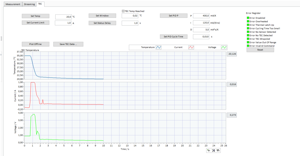
Figure 33: TEC window after pressing "Plot Online" and enabling TEC
