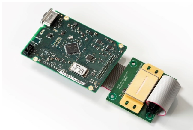
Figure 8: Evaluation Board connected via the ribbon cable and the adapter board to the PbS Array Module
